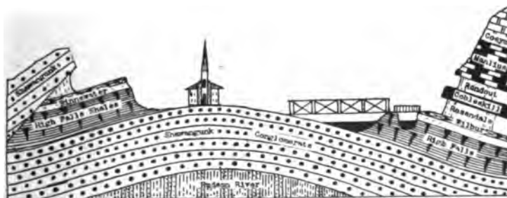
FIG. 1179. — Section across the pitching anticline at Rosendale, New York, showing the unconformable relation of the Shawangunk conglomerate to the Hudson River shales and sandstones, the succeeding lower Monroe (High Falls) shales, Binnewater sandstone (middle Monroe) and the upper Monroe limestones. The two waterlimes have here been extensively quarried. On the left the Shawangunk conglomerate is brought above the Rosendale by a thrust fault. (Original.)
